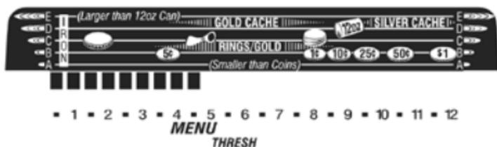
Press the MENU touch pad to display THRESH on the screen (above, with factory setting indicated on Upper Scale), and you can use the + and - touch pads to adjust the threshold of sound that is being produced by the GTI 1500 as it scans. Multiple touches will increase or decrease the level. Changes can be seen on the Upper Scale.
