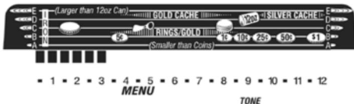
After using the MENU touch pad to display TONE on the screen, the factory tone setting will be indicated on the Upper Scale, as shown. Use the + and - touch pads to adjust the audio to preferred pitch or tone. Touching the + pad will raise the tone into a higher treble range, while touching - will
